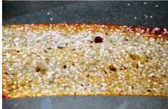
Figure 11. Sand grains 15%, Northern Region, Chiangyan Temple Sample 1, PPL magnification 10x.
