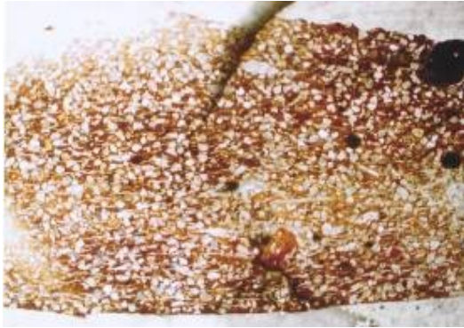
Figure 7. Sand grains 10-20%, Ancient Khitkhin Sample 2, PPL magnification 10x.
