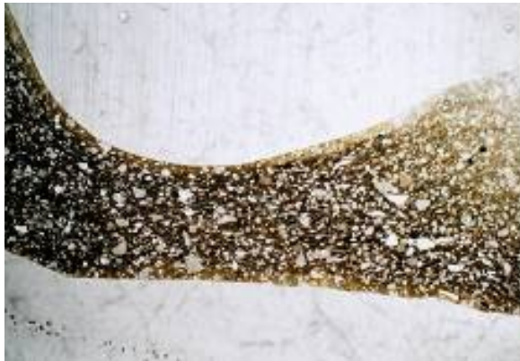
Figure 18. Sand grains 20-25%, Ancient Sema Sample 3, PPL magnification 0.75x.
