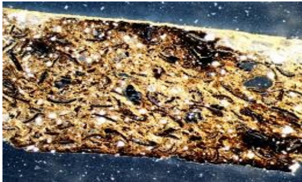
Figure 16. Ancient Sema Sample 5, Northeast Region, XPL magnification 2.5x.
