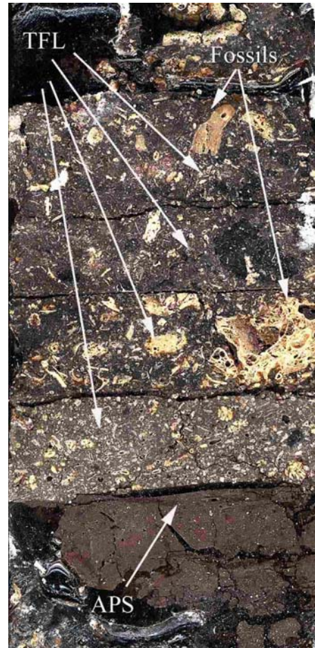
Figure 2: Scan of 15 cm long impregnated block (M18) that sampled Layer 5 – a plant-tempered adobe preparation surface (APS), and Layer 6 – a series of fossiliferous tufa floor layers (TFL) composed of quarried slabs of tufa; the basal slab and overlying thicker slabs showing natural horizontal splitting. Tufa is a type of limestone formed in calcareous springs.
