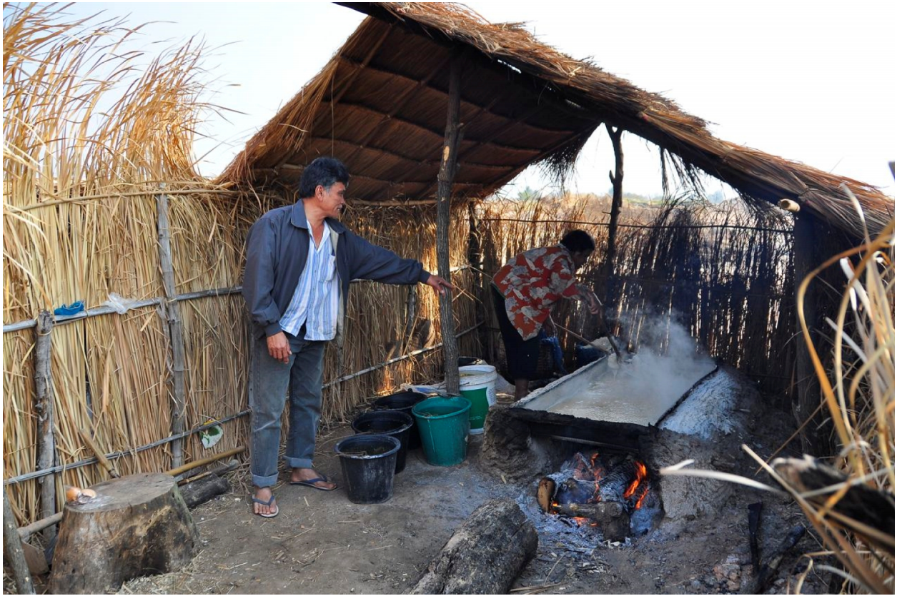
Figure 3: Evaporating brine water – Ban Don Phangat, Nakhon Rachasima Province.
