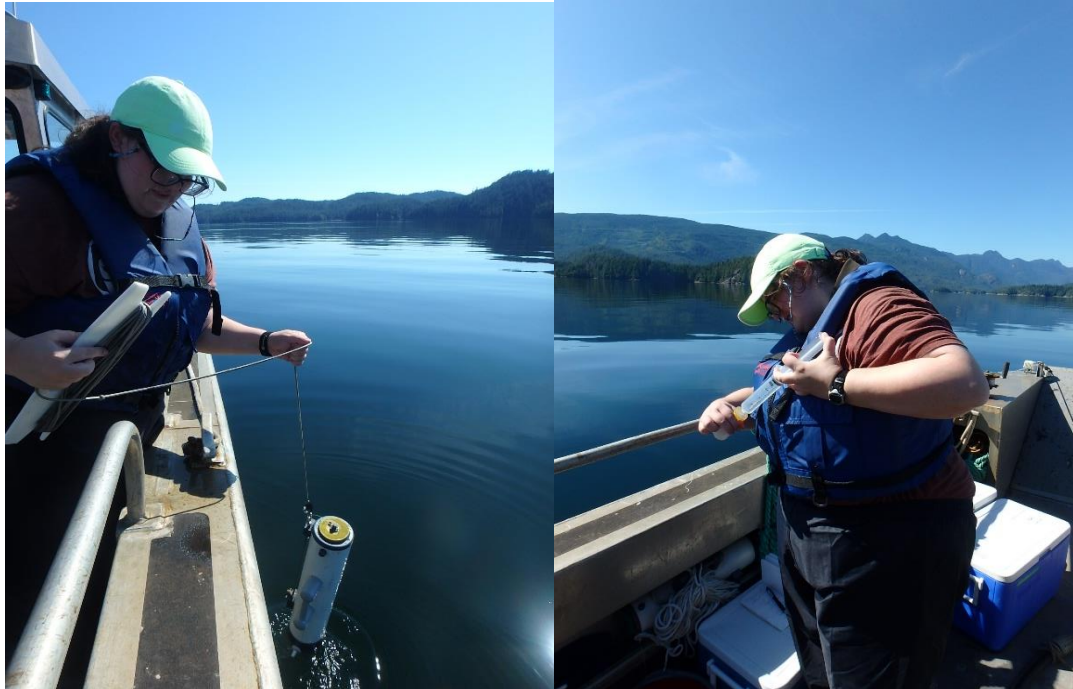
Figures 2a & 2b. Field sampling on the R/V Beach Hopper in Clayoquot Sound, BC, Canada, September 2024. Figure 1 shows a triggered Thoreson bottle being hand-hauled into the boat. Figure 2 shows nutrient samples being syringe filtered into a sample bottle.
