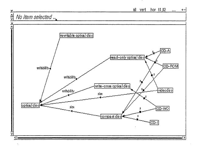
Figure 4. A CODE4 visibility mask applied to a graphical browser. Only those concepts having the value 'disc' for the property 'physical form' are displayed.
